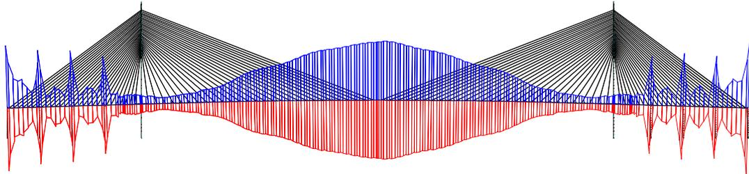
Figure 6: Bending moments of the bridge deck
