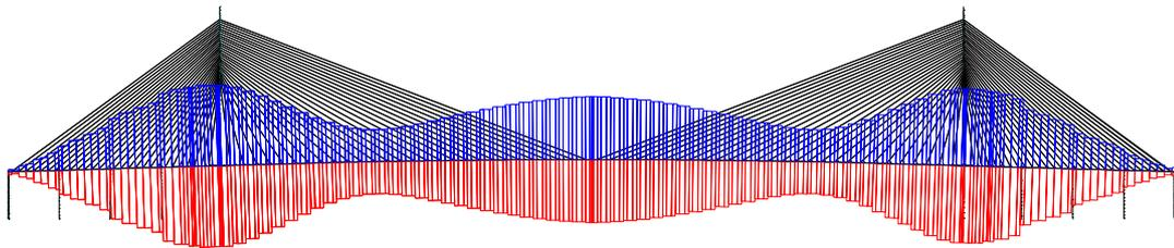
Figure 7: Normal forces in the bridge deck
