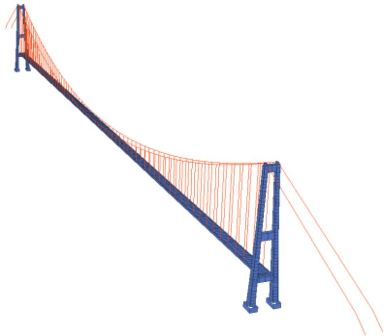
Fig. 4 Structural model of Hardanger bridge.
