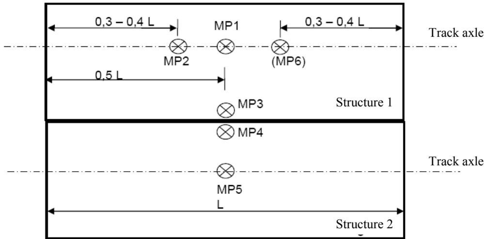
Figure 4. Measurement layout for a single span bridge
