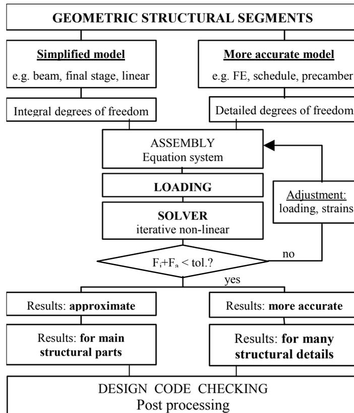
Fig. 3 Flow chart of hybrid FE analysis
