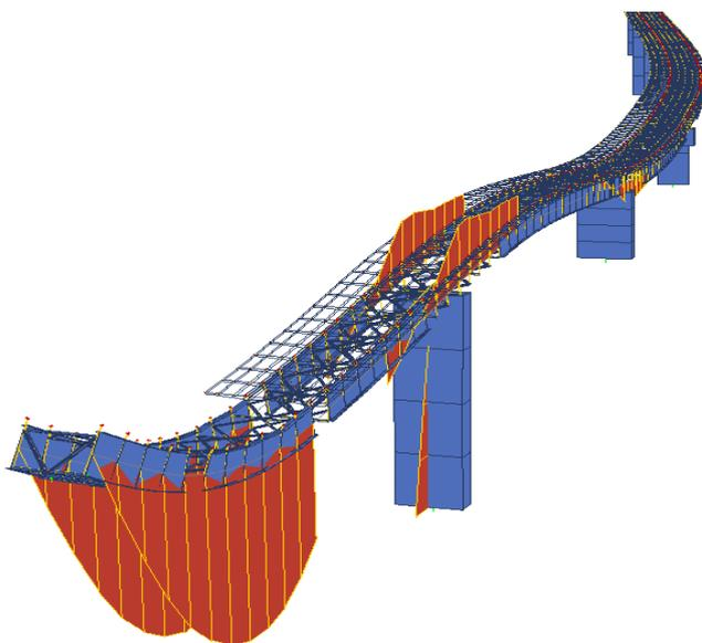
Fig. 9 Composite bridge in construction stage - integral results in real and virtual beams
