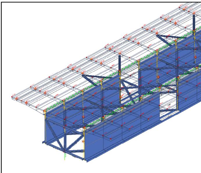
Fig. 1 Typical hybrid model of the bridge with beam steel members and “virtual” beam slab implemented as substructure with shell elements
