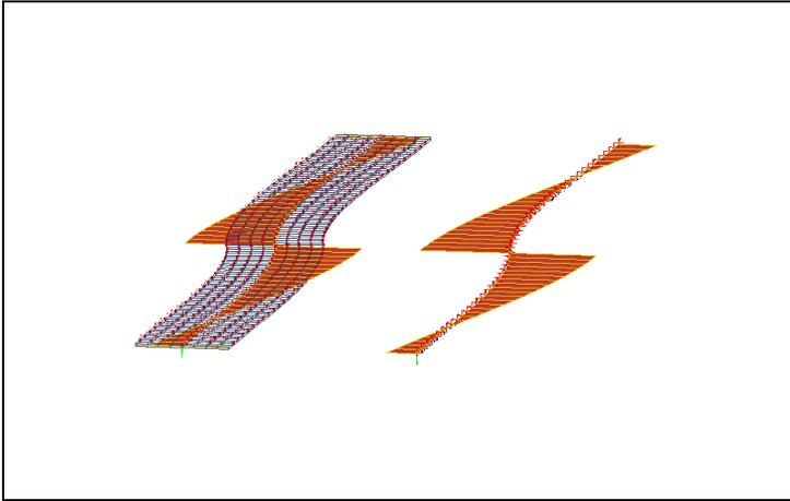
Fig. 4 *In plane moment applied as a loading to the plate bridge modelled with shell elements*
