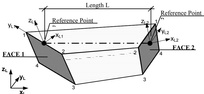
Fig. 2 Structural segments defined by the length, and the face geometry at begin and end
