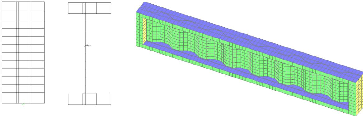
Fig. 5 Cross-sections and calculation model of a girder with corrugated steel web
