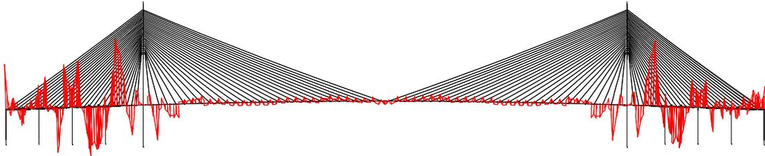
Figure 9. SCB - Construction stages analysis (without creep and shrinkage).
