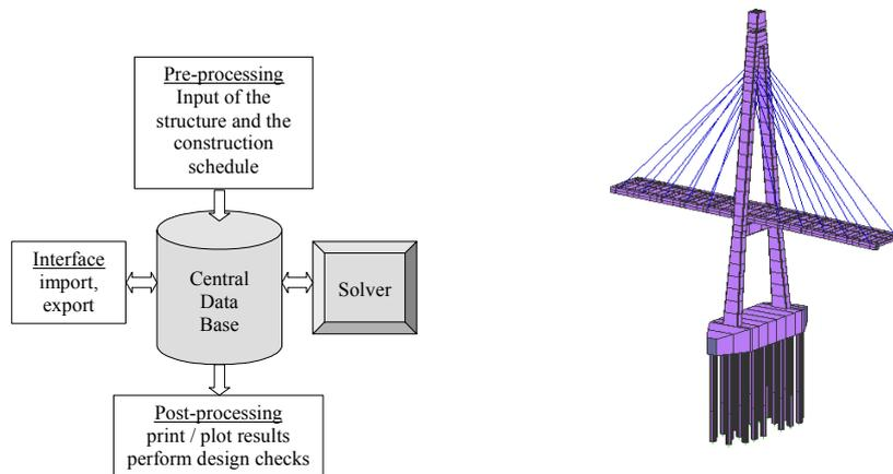
Figure 7: Structure of the bridge design software *RM2000/RM2004* with visualisation example
