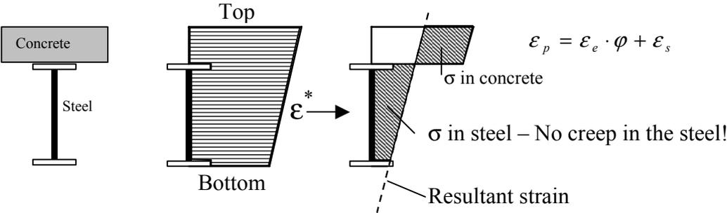
Figure 5: Primary effects in concrete/steel composite section
