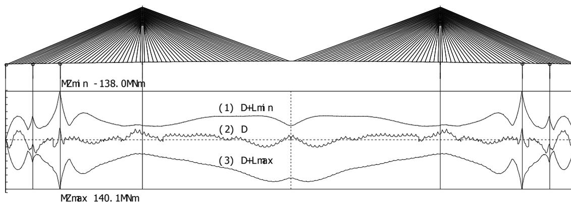
FIGURE 8 – BENDING MOMENT ENVELOPE IN DECK
