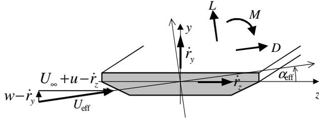
FIGURE 7 - CONTRIBUTIONS TO EFFECTIVE VELOCITY FOR BUFFETING ANALYSIS
