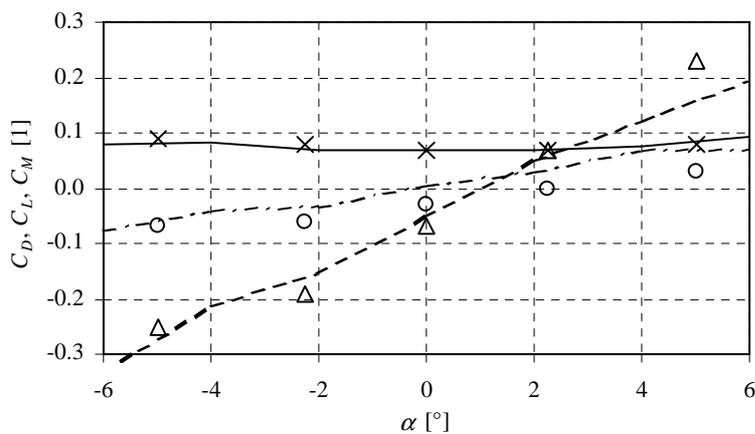
FIGURE 4 - STEADY STATE COEFFICIENTS  $C_D$  (SOLID LINE, X),  $C_L$  (DASHED LINE, O) AND  $C_M$  (DASH-DOTTED LINE,  $\Delta$ ) FOR STONECUTTERS BRIDGE, RESULTS MARKED WITH SYMBOLS ARE DVMFLOW RESULTS
