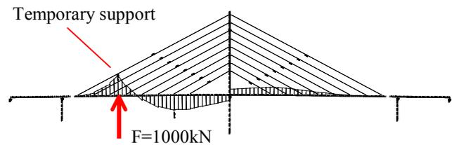
Fig.10 Bending moments on the main girder before closure (with temporary primary support active)
