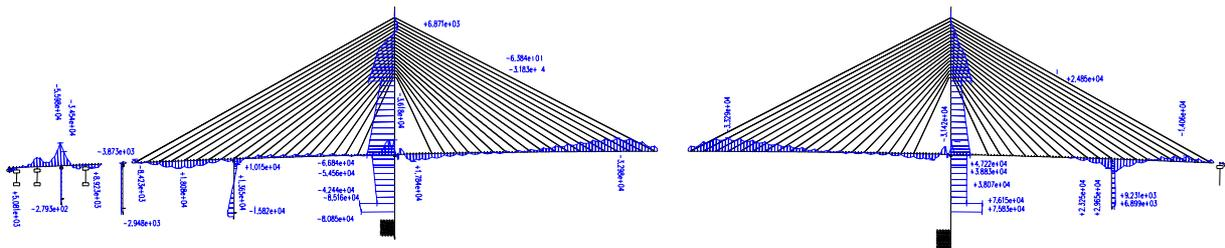
Fig.16 Construction stage 71 after closing of the approach spans 2 and 3, bending moments in the superstructure
