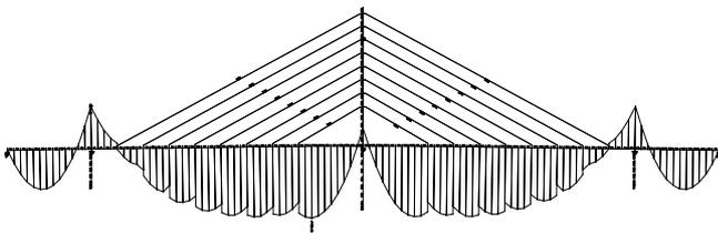
Fig.1 Bend. Moment  $M_z$  at final stage without optimisation
