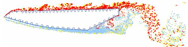
**Figure 7 - Typical flow pattern of Vortex particles around cross section**
