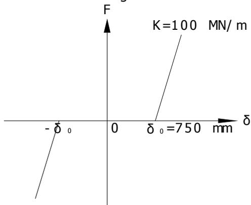
**Figure 11 – Static force-displacement relationship of the dampers**
