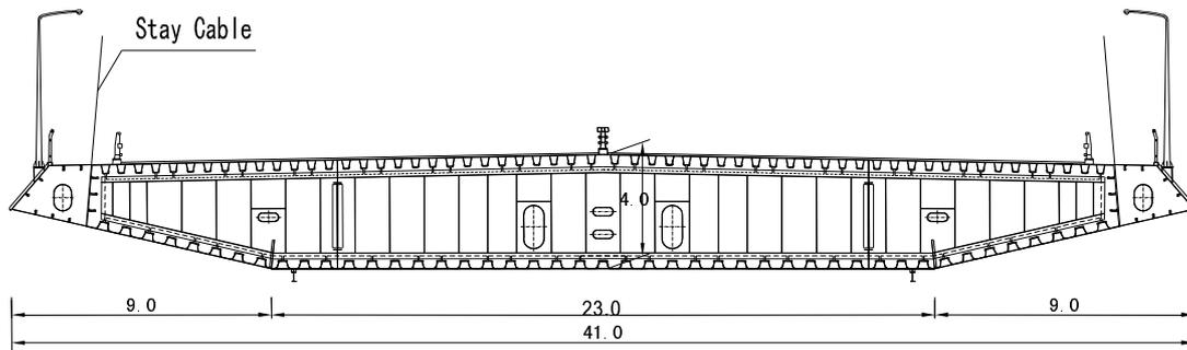
**Figure 3 – Sutong Bridge - Cross-section of the Girder [m]**
