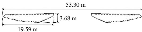
**Figure 6 - Twin girder system of Stonecutters Bridge**
