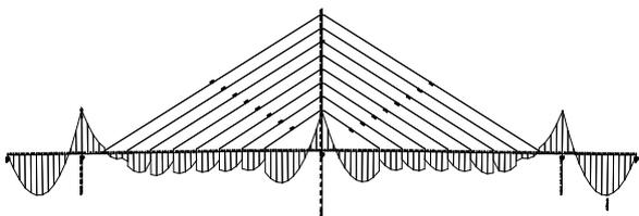
**Figure 4 - Target bending moment to be achieved with construction sequence**
